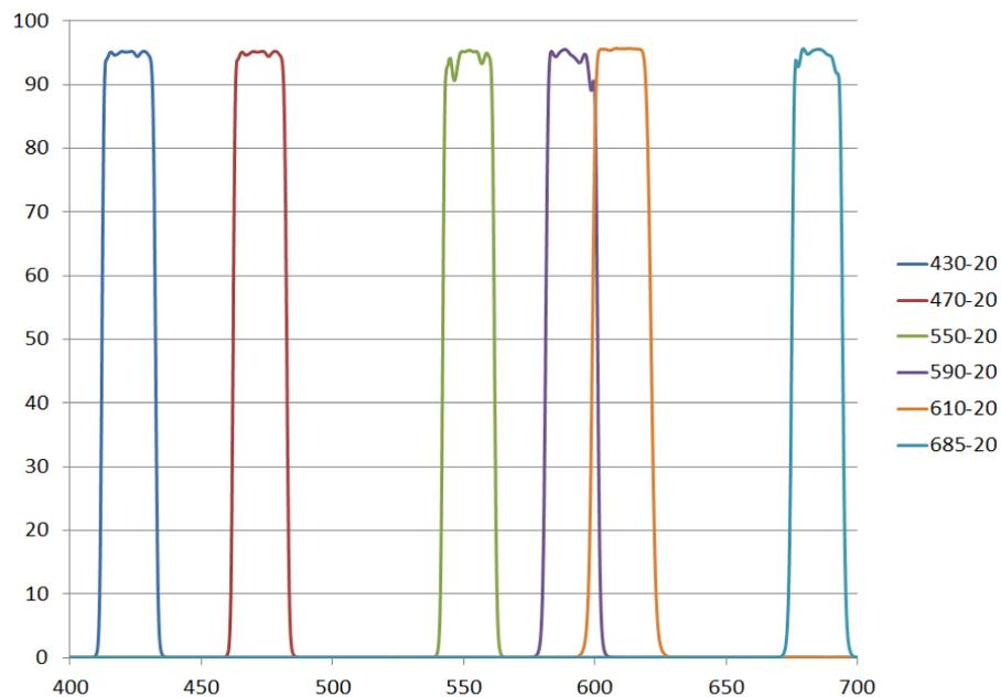
**Fig. 3** Hard coatings by Alluxa on a single side of a glass substrate. Note that with an AR on the back the transmission would approach 100%. Also note the inherent improved "squareness" of spectral shape, which helps S/N by increasing transmission as well as blocking. Improved shape is direct result of the repeatability of automation.
