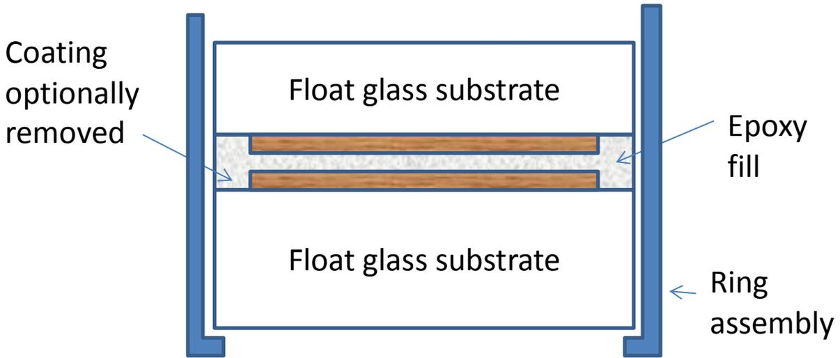
**Fig. 1** A typical soft coating has three structures laminated together to help provide moisture resistance. The structure is typically 2-5mm in thickness and mounted in a ring to further try to restrict humidity ingress.
