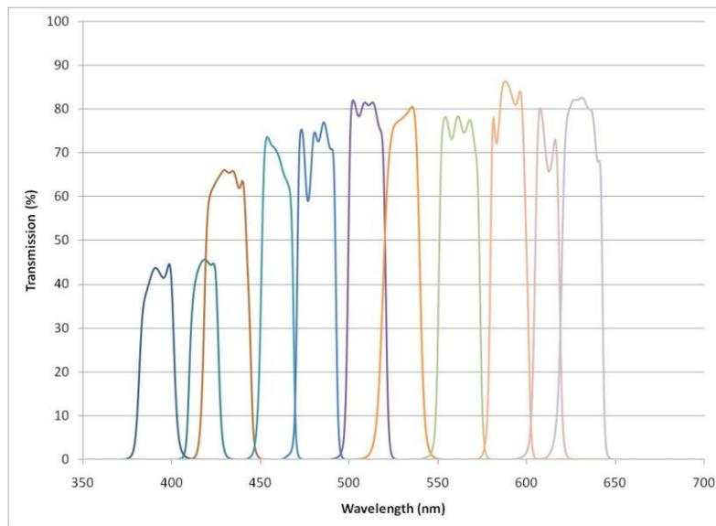
**Fig. 2** Soft coating designed for high transmission that contains no silver layers. The transmission can rise above 80% in the green/red, but drops to less than 50% in the UV blue. Also note the severe ripple in the pass-band attributable to the lack of computer controlled deposition control.
