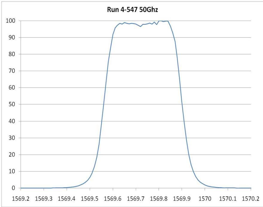
**Fig. 5** Ultra-narrow band filter built using Alluxa's plasma deposition technology. The bandwidth is approximately 0.3 nm in bandwidth at 1570nm.
