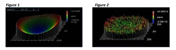
Figure 1 shows a flatness measurement of a dichroic coated with a standard hard coating process. Figure 2 shows the same dichroic coated using Alluxa's very low stress process.
