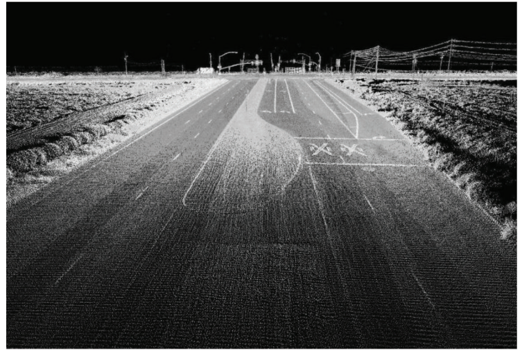
Figure 2: LIDAR data point cloud showing a detailed 3D street view. Image credit: Oregon State University
